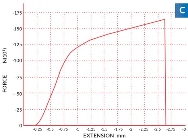
A: zirconia sample. B: PEEK sample. C: base metal sample. Note the fragile behavior of Zirconia compared to the plastic nature of base metal extending the fracture limit to its most. The PEEK samples illustrated an intermediary behavior.
