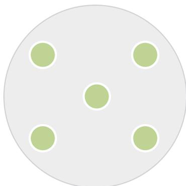
The five areas where the thickness of the biofilms was measured using a micrometer are shown (Mitutoyo Digimatic 1”).
